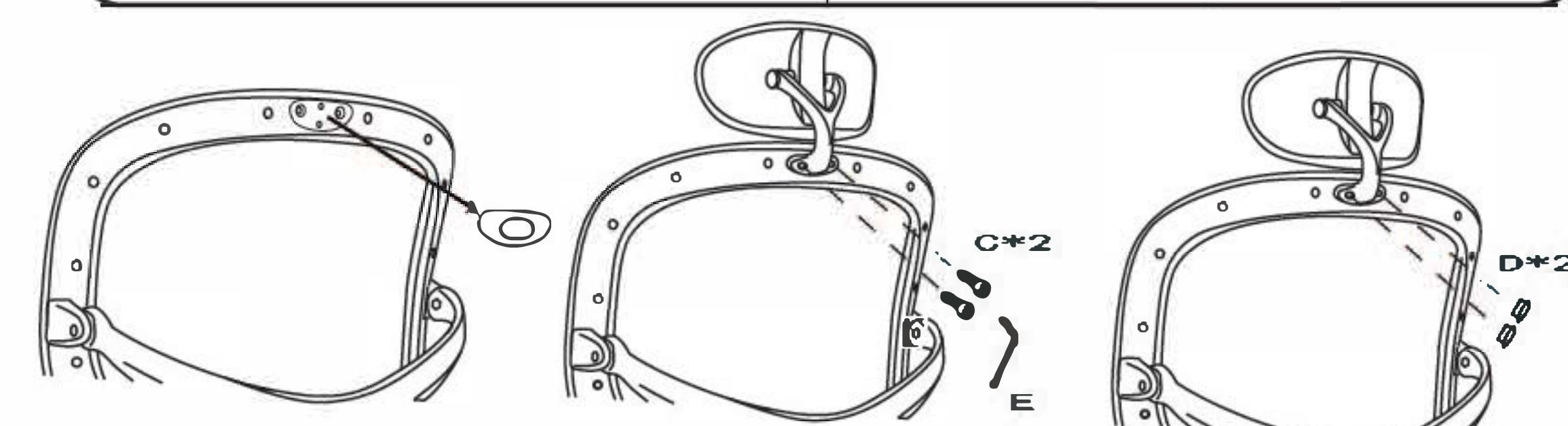
1. Remove the plastic cover on the back.
